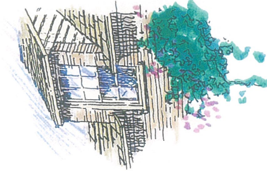
▲ Shed roof dormer penetrating roof plane.
